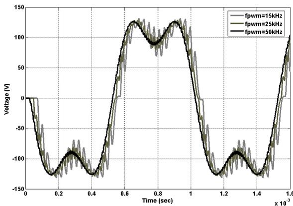
Fig.2: Voltage waveforms applied to  $R_{lamp}$  for different  $f_{pwm}$
