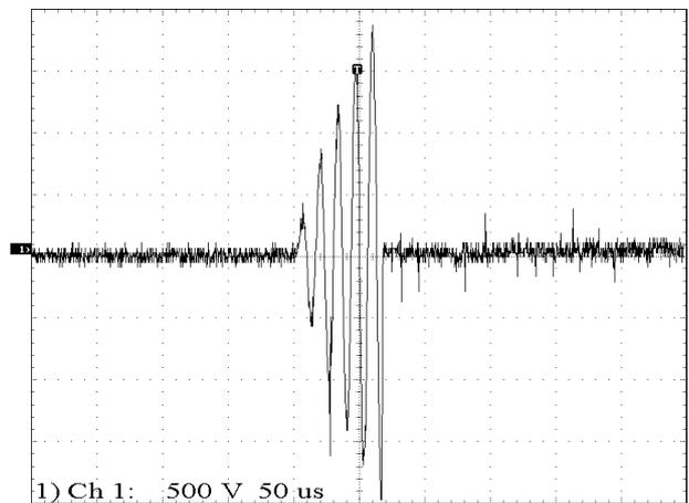
Fig. 11: Measured lamp voltage waveform in ignition
