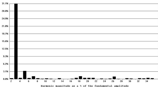
Fig 14: Harmonic spectrum of current with  $f_{pwm} = 32768\text{Hz}$
