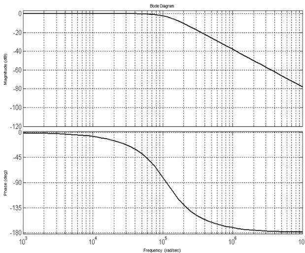
Fig. 6 : Frequency response of the designed LC filter,  $L=833\mu H$ ,  $C = 92nF$  e  $R_{lamp} = 66.6\Omega$ .
