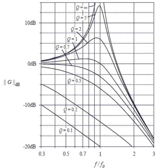
Fig. 4: Filter gain versus frequency for different values of  $Q$
