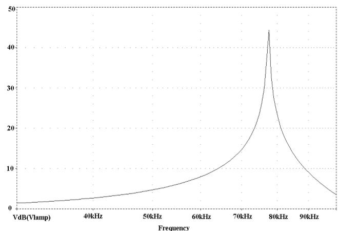
Fig. 7: Frequency response of filter ( $LC_{ig}$ )
