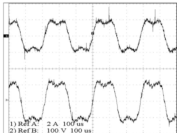
Fig. 12: Measured lamp voltage and current waveforms
