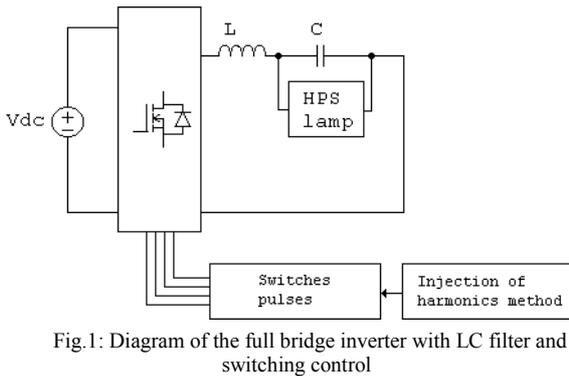
Fig.1: Diagram of the full bridge inverter with LC filter and switching control
