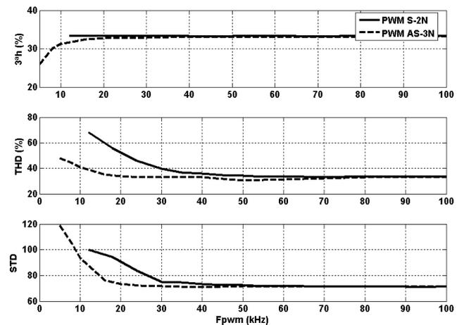
Fig.3 : a) Third harmonic current amplitude, b) THD of the current and c) STD of the power
