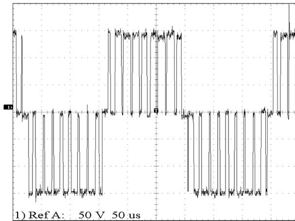
Fig. 16: Inverter voltage waveform
