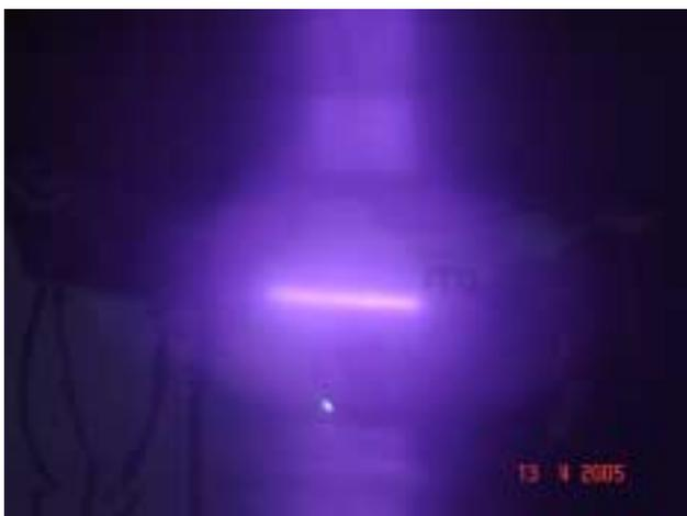
Fig 15: Picture of the arc path of the lamp operating at fundamental frequency of 3.5kHz
