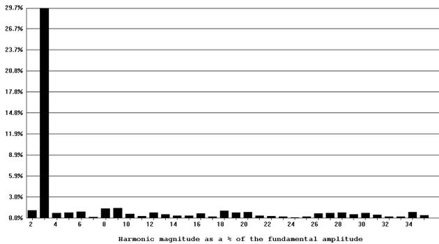
Fig 13: Harmonic spectrum of current with  $f_{pwm} = 32768\text{Hz}$
