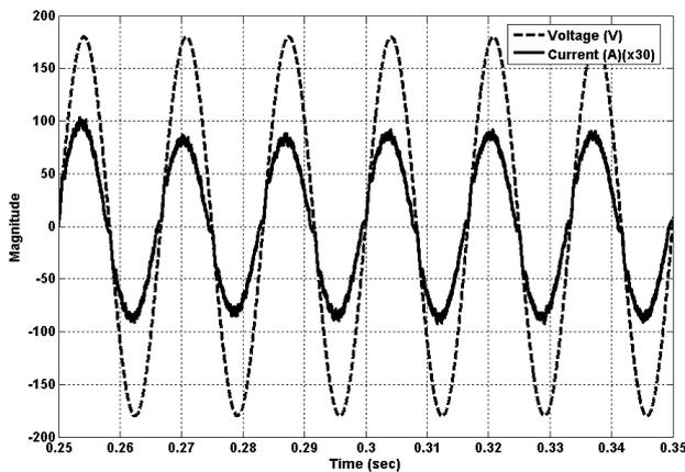
Fig. 9: Line input voltage and current waveform
