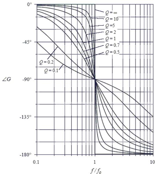
Fig.5: Filter phase versus frequency for different values of Q
