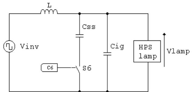
Fig. 7: Scheme of the ignition circuit
