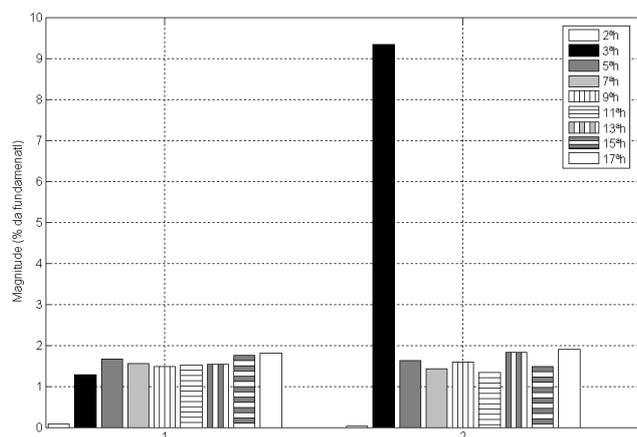
Fig. 10 :Spectrum of the input current for methods 1 (120Hz sampling) and 2 (ordinary)
