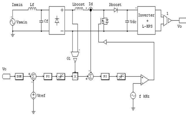
Fig.8 : Complete diagram of the electronic ballast emphasizing the power factor corrector (PFC) and control loops
