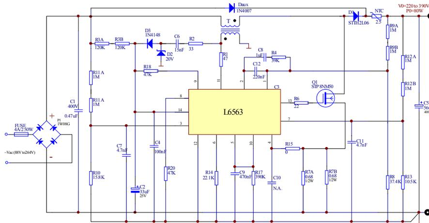
Figure3. The high active power factor correction circuit of the electronic ballast for 80W high-pressure sodium lamps based on L6563
