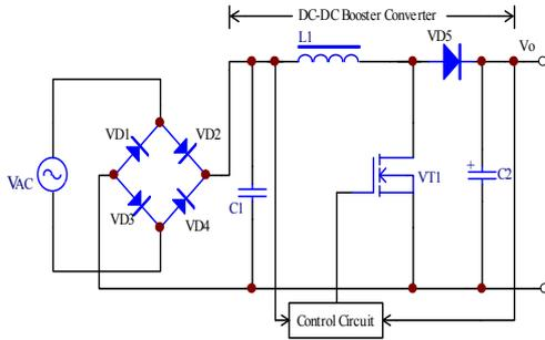
Figure2. The basic framework of APFC circuits
