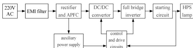
Figure1. Schematic diagram of HPS electronic ballast
